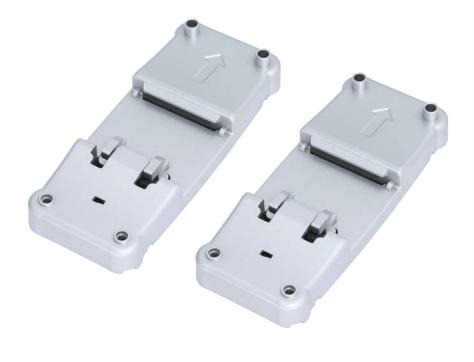
Victoria, BC, Canada – The MP-DINRAIL is a two piece ABS adapter that is custom designed to convert the standard MACH-ProCom, MACH-ProSys, MACH-ProPoint, and MACH-Pro1/2 enclosures to be DIN rail mountable. Adapter kits use the standard #8 TEK screws that ship with the controllers to fasten the adapter to the enclosure.
